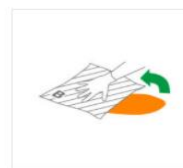
Push down onto side B, which is plastic backed, and wipe until spill is fully absorbed.
