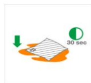
Place the active side (A) face down onto the spill. Leave to absorb for 30 sec.
